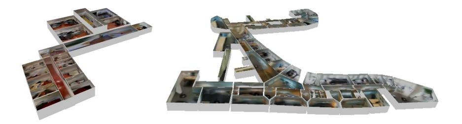
3D reconstruction of a 655 mq office with 19 rooms. This environment was acquired with a mobile phone (HTC One M8)
